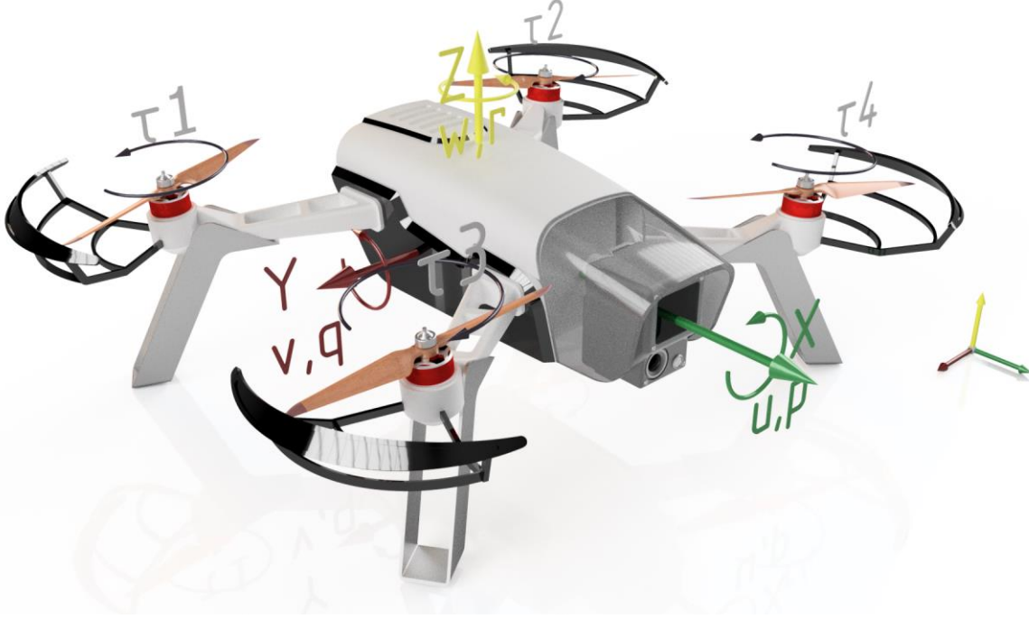
Fig. 1. Inertial and body reference frames, flight configuration “x”, a simplified design [2]
